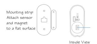
Battery receptacle Contains one CR2032 3V lithium battery
